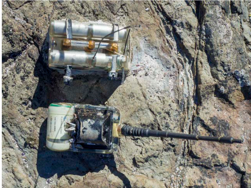
Figure 4 - The satellite tags. Top: the Wildlife Computers tag (1), bottom; the SMRU tag (2).
